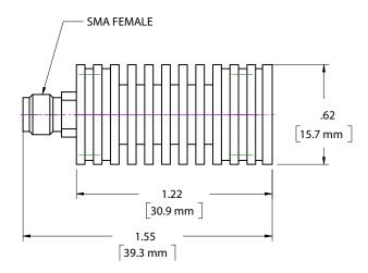
Compact design for low size/power ratios. Designed to meet MIL-DTL-3933 environmental specification.
