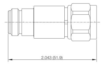
Drawing not to scale. Dimensions for reference only Units: inches (mm)
