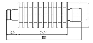
Drawing not to scale. Dimensions for reference only Units: mm
