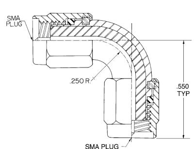
VSWR and Frequency Range Specifications are for reference and are dependant on cable type and other application specific conditions
