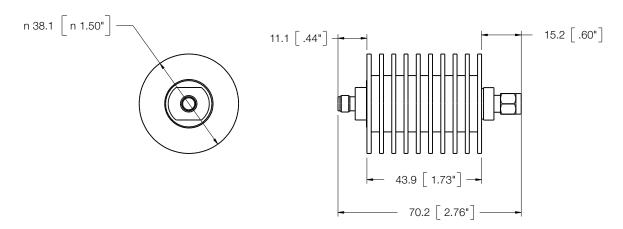
Designed to comply with MIL-DTL-3933
